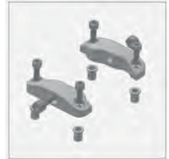
Fastening of frame sections for units of sizes greater than 32 (Fig. 7.1.)
